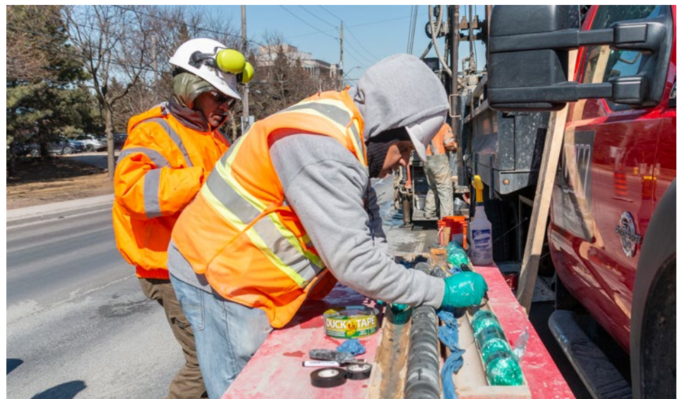
Examining soil samples during preliminary engineering on a Yonge Street project.
